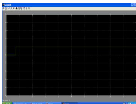
Fig 16: This is the b output of Bang-Bang phase detector. Output b = c only when there is a phase shift due clock late
