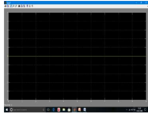
Fig 13: This is the b output of Bang-Bang phase detector. Output b = c only when there is a phase shift due clock late. Here its how zero output because there is no phase shift.
