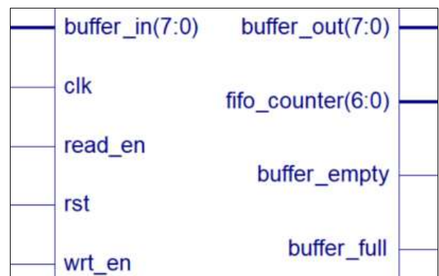
Fig 1: RTL Schematic of FIFO buffer
