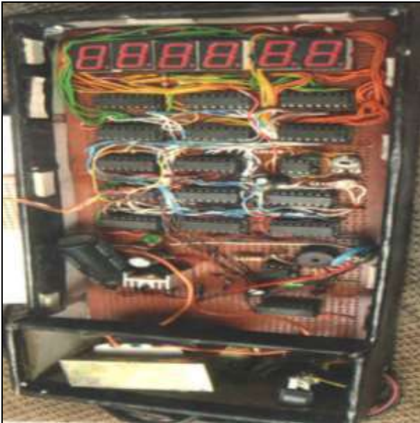
Fig 7: Hardware Internal circuitry of digital clock with hourly alarm
